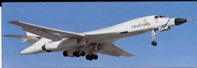
Above: Unusually, the first flight of the prototype B-1A was also the first flight of the YF101 turbofan. New engines are more often tested in an existing airframe before being flown in a new aircraft type.
